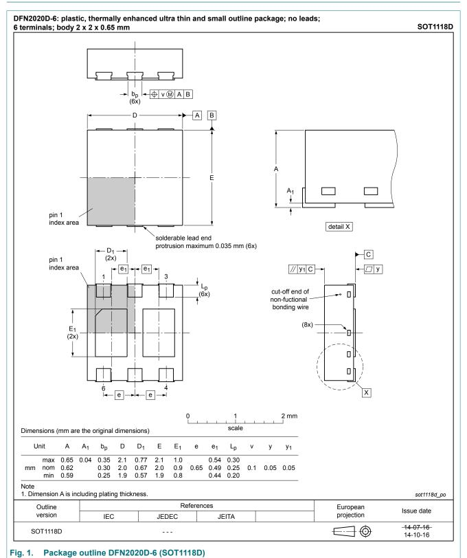
plastic, leadless thermally enhanced ultra thin and small outline package; 6 terminals; 0.65 mm pitch; 2 mm x 2 mm x 0.65 mm body
